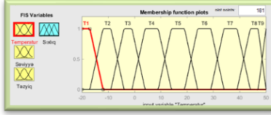
Figure 5. Graphical representation of the membership functions for the input linguistic variable - temperature of the oil product
